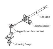
1-Input / 2-Output Mechanism
